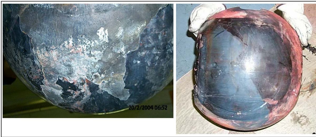
Figure 12 – Photographs of the Ball Surfaces with Cr 2 O 3 -blend Coating (left) and with n-TiO 2 Coating (right) after Same Service Exposure and Conditions
