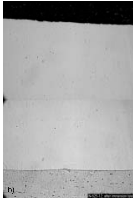
Figure 6. Inconel 625 coatings after corrosion test in 3.5 % NaCl. a) HVOF coating and b) laser coating.
