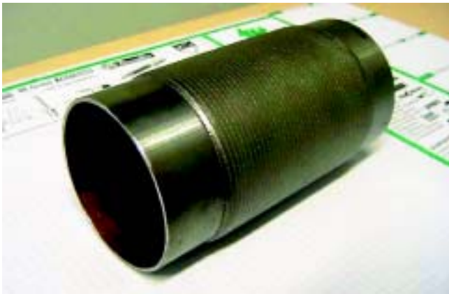
Figure 9. Thin walled (2 mm) stainless steel tube with a laser coating (Photo: Fortum Service Oy Laser Coating Centre).
