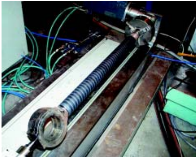
Figure 12. Laser coated hydraulic piston. The piston was laser coated by using a high rate 6 kW HPDL laser coating process with a corrosion resistant coating (Photo: Laser Application Laboratory, Tampere University of Technology).
