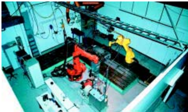
Figure 13. Overview of the Laser Application Laboratory (LAL, Tampere University of Technology). Two high power lasers (6 kW HPDL, 4 kW Nd:YAG) are used for surface hardening, laser coating and for laser welding research and development. Centre: HPDL with robot; bottom: powder feeder; left: power supply for HPDL; right: Nd:YAG with robot.
