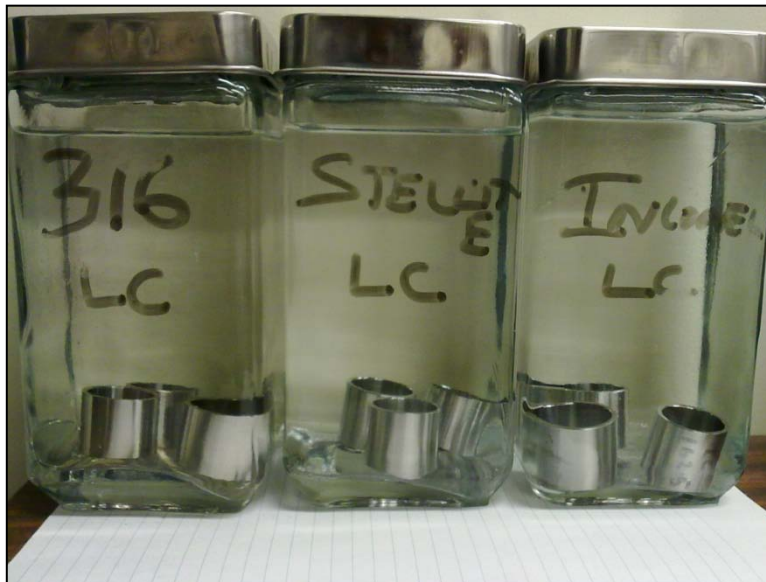
Fig. 3: Gravimetric test continuous exposure setup
